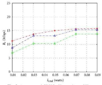
**Fig. 8.** Average total CRU Rs Vs. maximum PU tolerable interference power total for =0.7.
